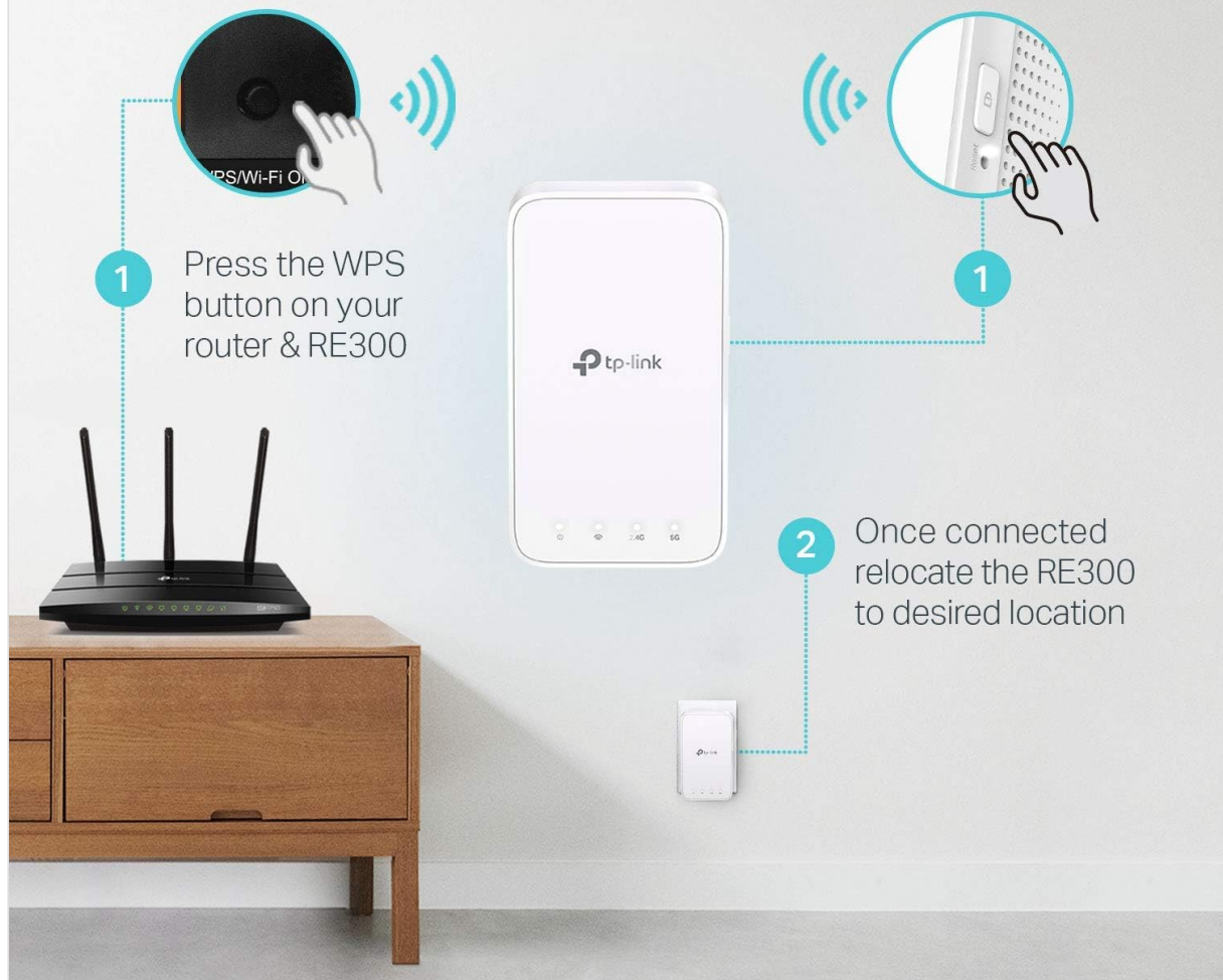
Image: Diagram showing how to set up the RE300 using the WPS button on both the router and the extender for a secure one-touch connection.
