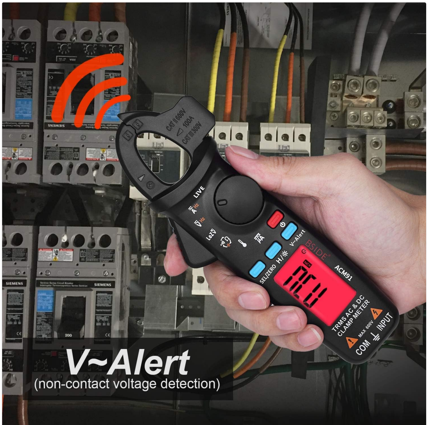
Figure 6.1: NCV (Non-Contact Voltage) detection in progress, showing the meter's ability to detect voltage without physical contact.
