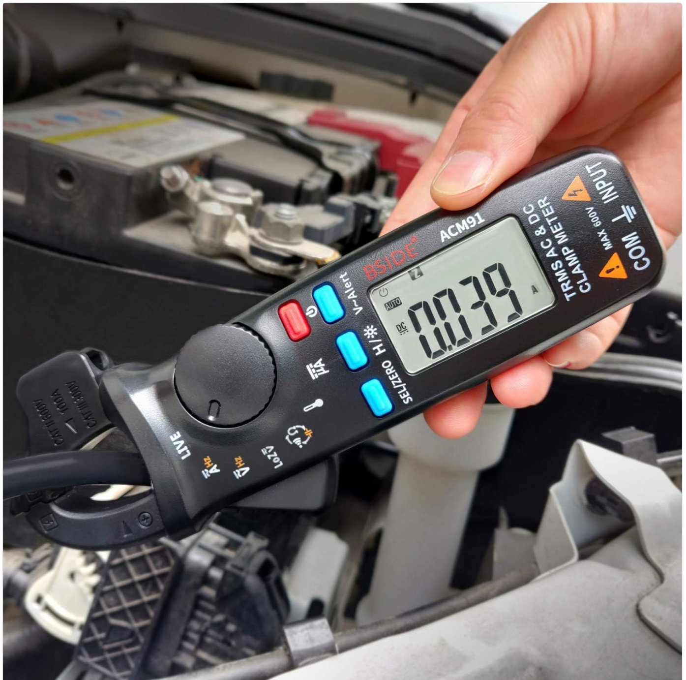
Figure 1.1: The BSIDE ACM91 Clamp Multimeter being used to measure current in an automotive application. The display shows a reading of 0.039 amps.
