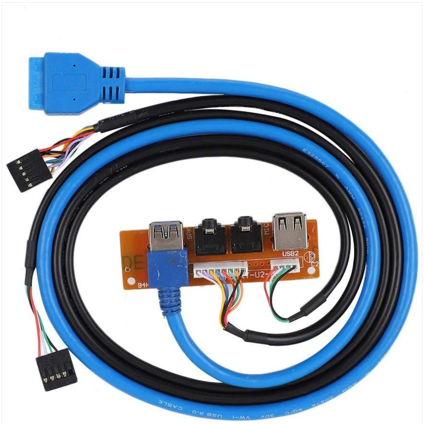
Figure 1: Overview of the Wendry Computer Chassis Front Panel, showing the main board with USB and audio ports, and the connected USB 3.0 and USB 2.0 cables.
