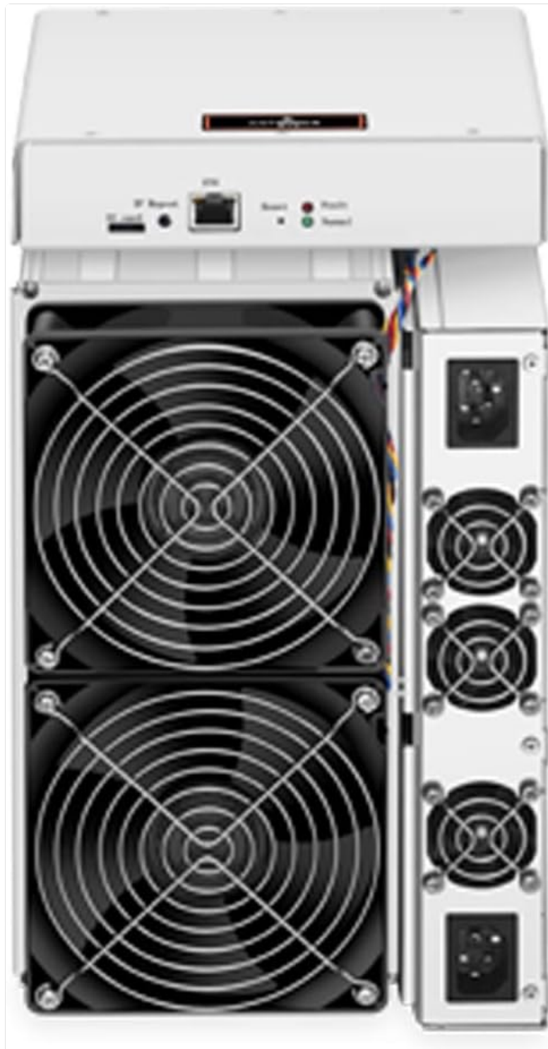
Figure 3.2: Detailed view of the Antminer T17+ front panel, showing the network port, indicator lights, and multiple power input sockets.
