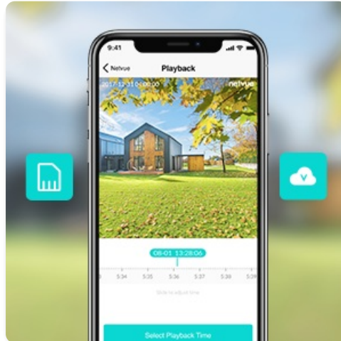
Image: The camera supports both local storage via an SD card and optional cloud storage for video recordings.
