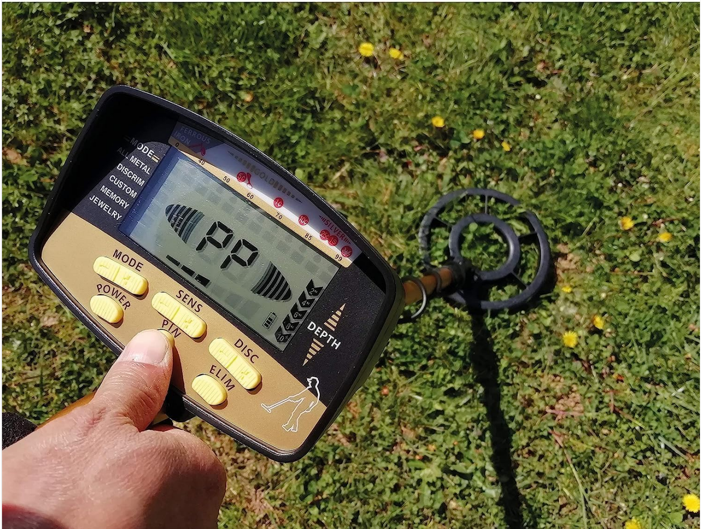
Image: A user's hand pressing the 'PIN' button on the S3800 control panel, with the LCD screen displaying "PP" to indicate pinpoint mode, aiding in precise target location.
