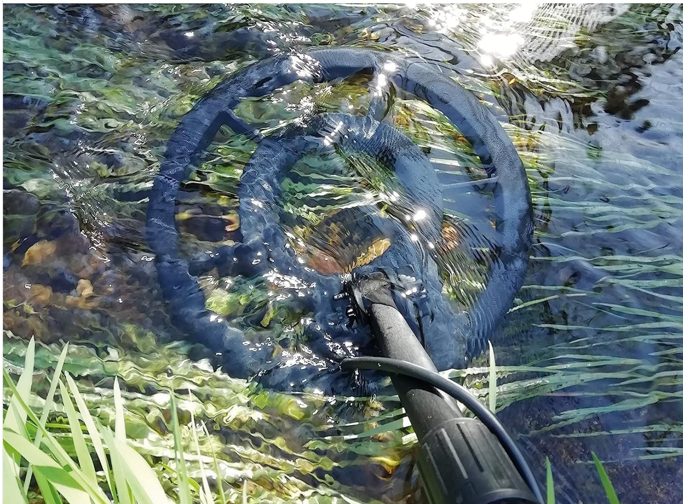
Image: The S3800's IP68 waterproof search coil partially submerged in clear, shallow water, demonstrating its capability for detecting metals in wet environments.
