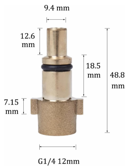
Figure 2.2: Detailed view of the adapter with key dimensions, including 9.4mm, 12.6mm, 18.5mm, 48.8mm, and G1/4 12mm, indicating its precise measurements for compatibility.
