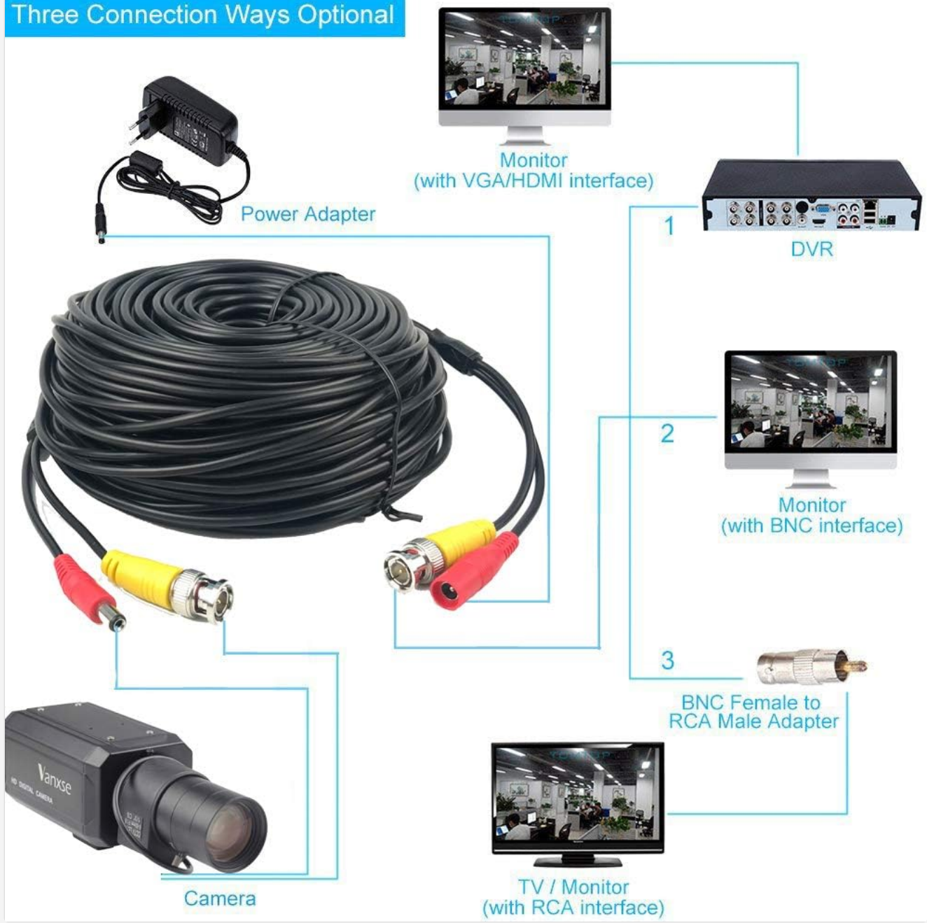
Figure 3.2: Three optional connection methods for the camera to various display devices.
