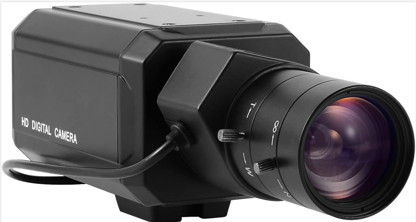
Figure 3.4: Varifocal lens with adjustable zoom and focus rings.
