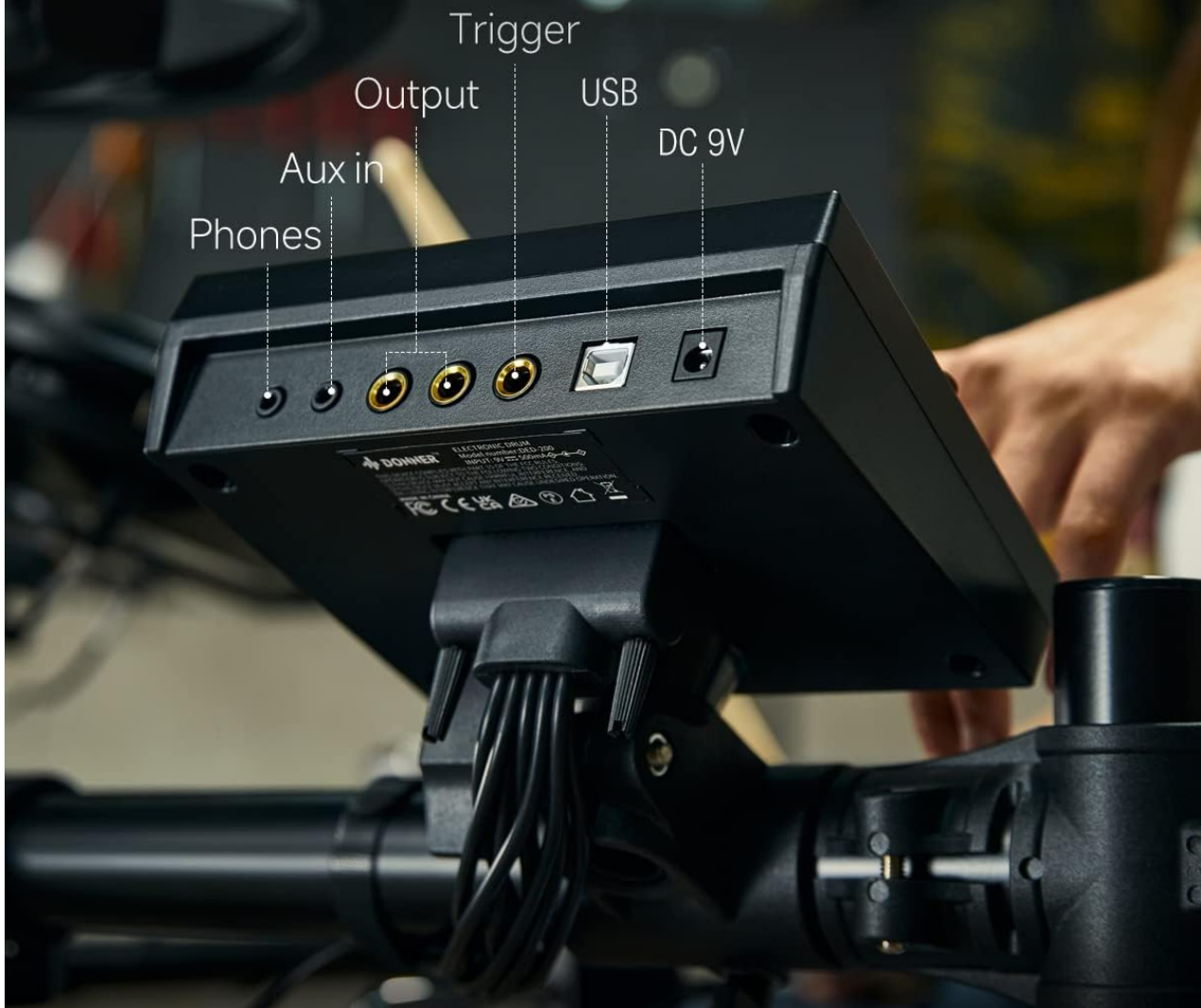
Figure 4.4: The rear panel of the DED-200 sound module, showing various input/output ports including Aux In, Phones, Output, Trigger, USB, and DC 9V power input.
