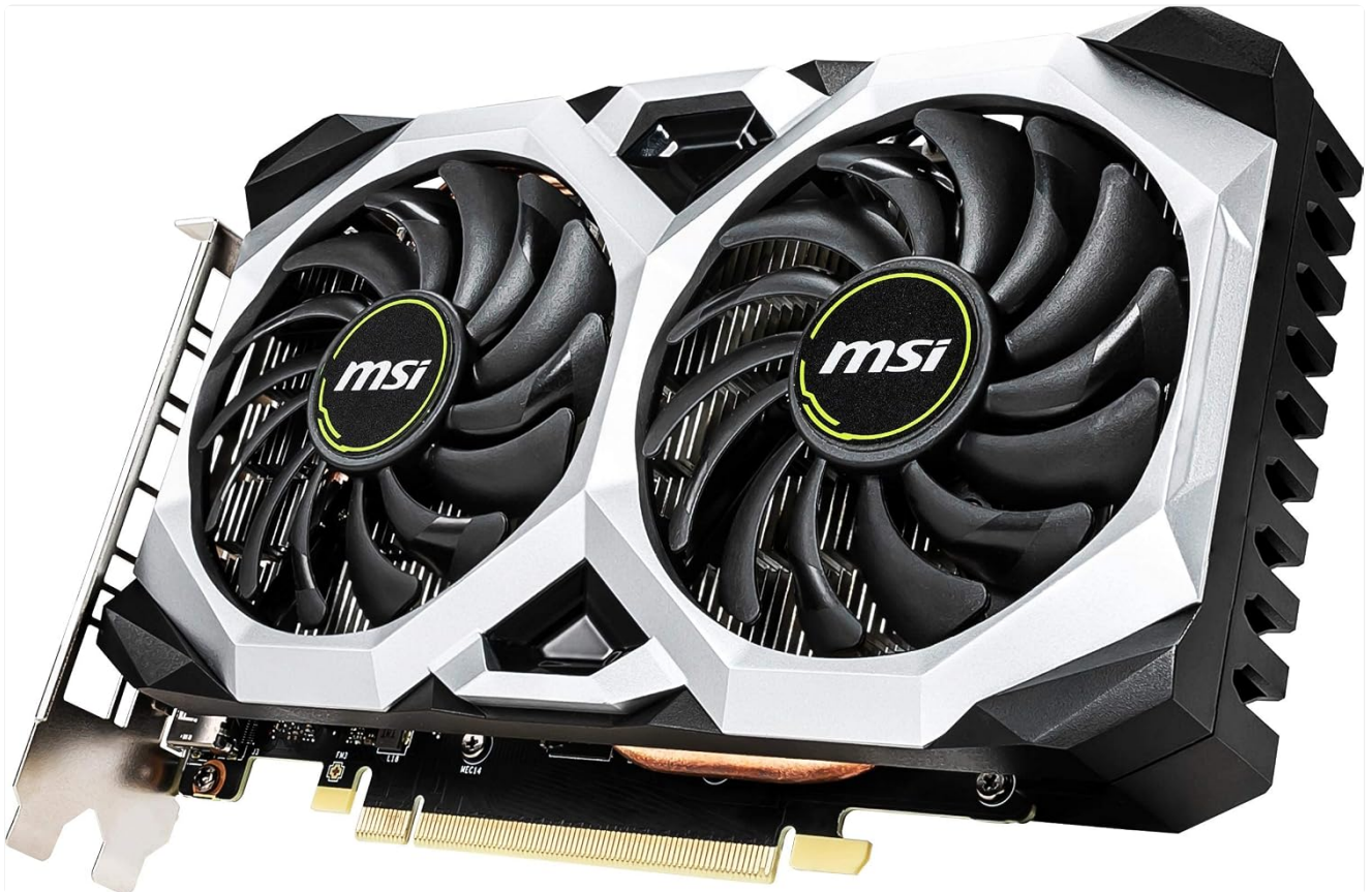
Image: Front view of the MSI GeForce GTX 1660 VENTUS XS 6G OC Graphics Card, showing the dual fans and heatsink assembly.
