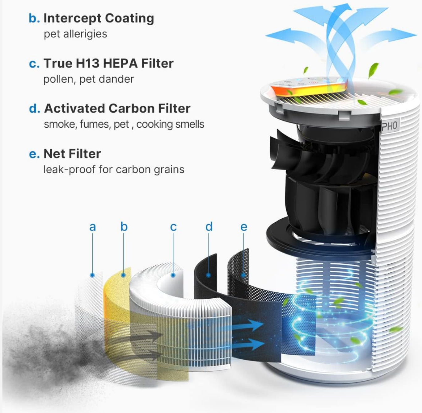
Image 1.2: Diagram illustrating the 5-stage filtration process of the RENPHO Air Purifier, including the Ultra-Fine Pre-Filter, Intercept Coating, True H13 HEPA Filter, Activated Carbon Filter, and Net Filter.
