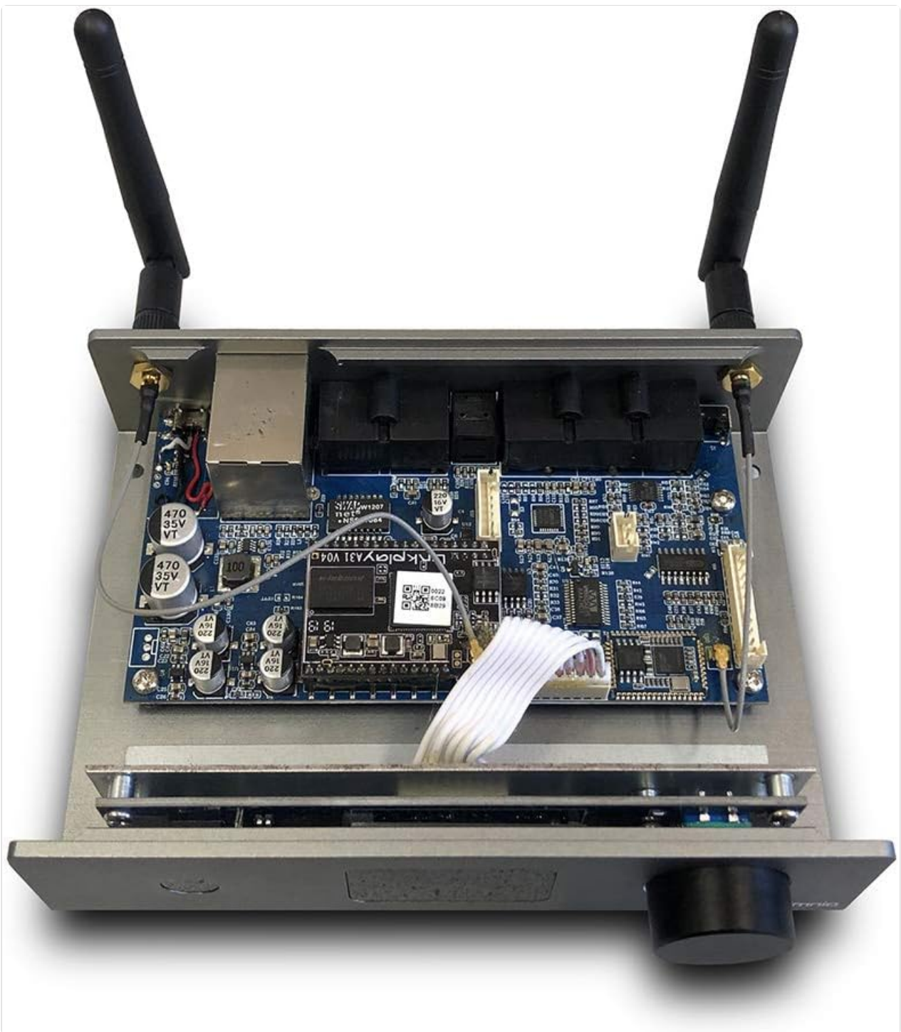
Figure 6.1: Internal view of the NuPrime Omnia WR-1, showing the circuit board and components. This image is for informational purposes only and does not indicate user-serviceable parts.
