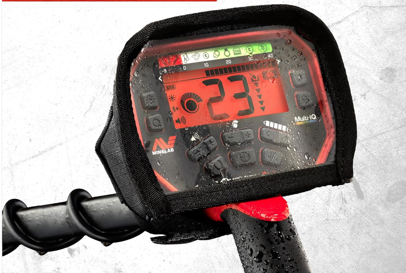
Image: The Minelab Vanquish 540 control unit protected by a rain cover, demonstrating its water-resistant design.
