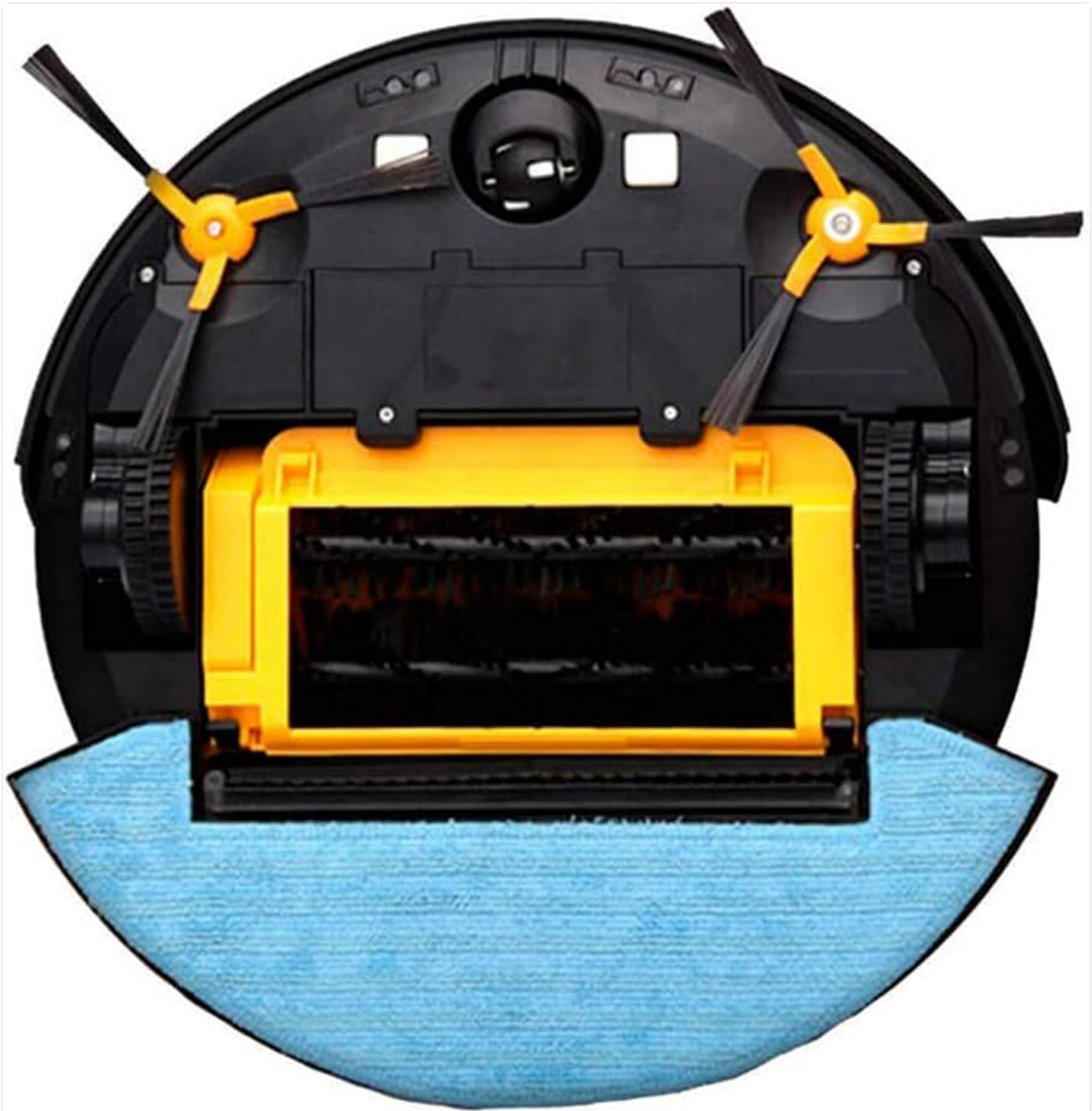
Image: Underside of the robot, displaying the two side brushes, main roller brush, and the attached mopping pad. The robot features dual side brushes, a central roller brush, and a mopping attachment for comprehensive cleaning.
