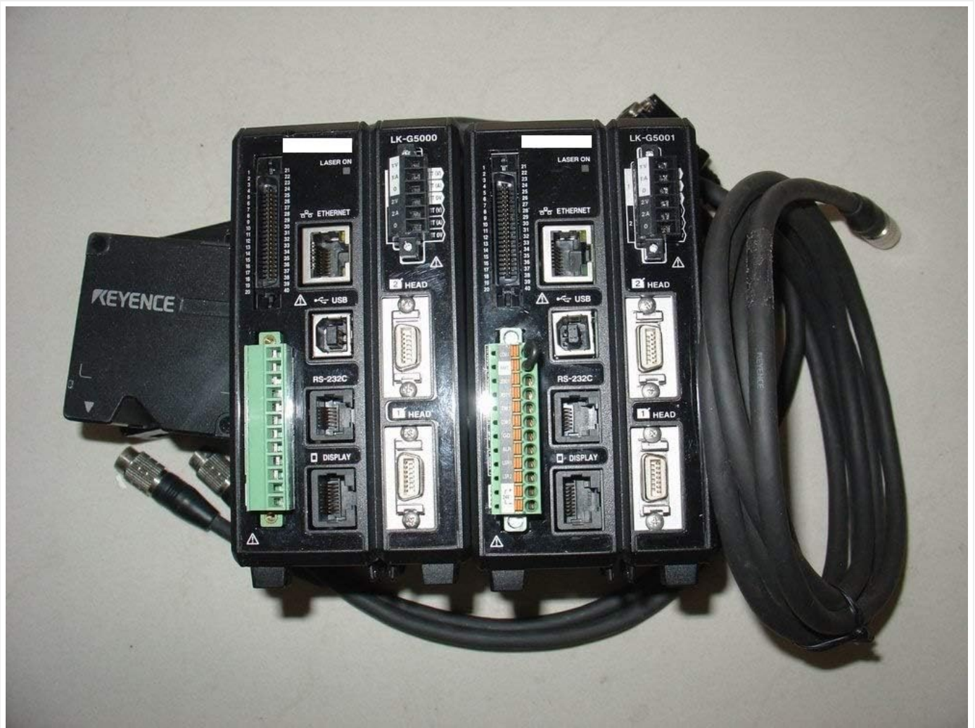
Figure 1: Overview of KEYENCE LK-G5001 and LK-G5000 series controllers. The image displays several black rectangular modules, including the LK-G5001, each with various ports and indicators. Visible ports include Ethernet, USB, RS-232C, Display, and multiple Head connections for laser sensors. Associated cables are also shown.
