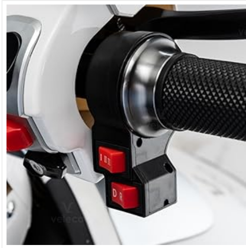
Figure 8: Close-up of the handlebar controls, including speed mode selector and reverse switch.
