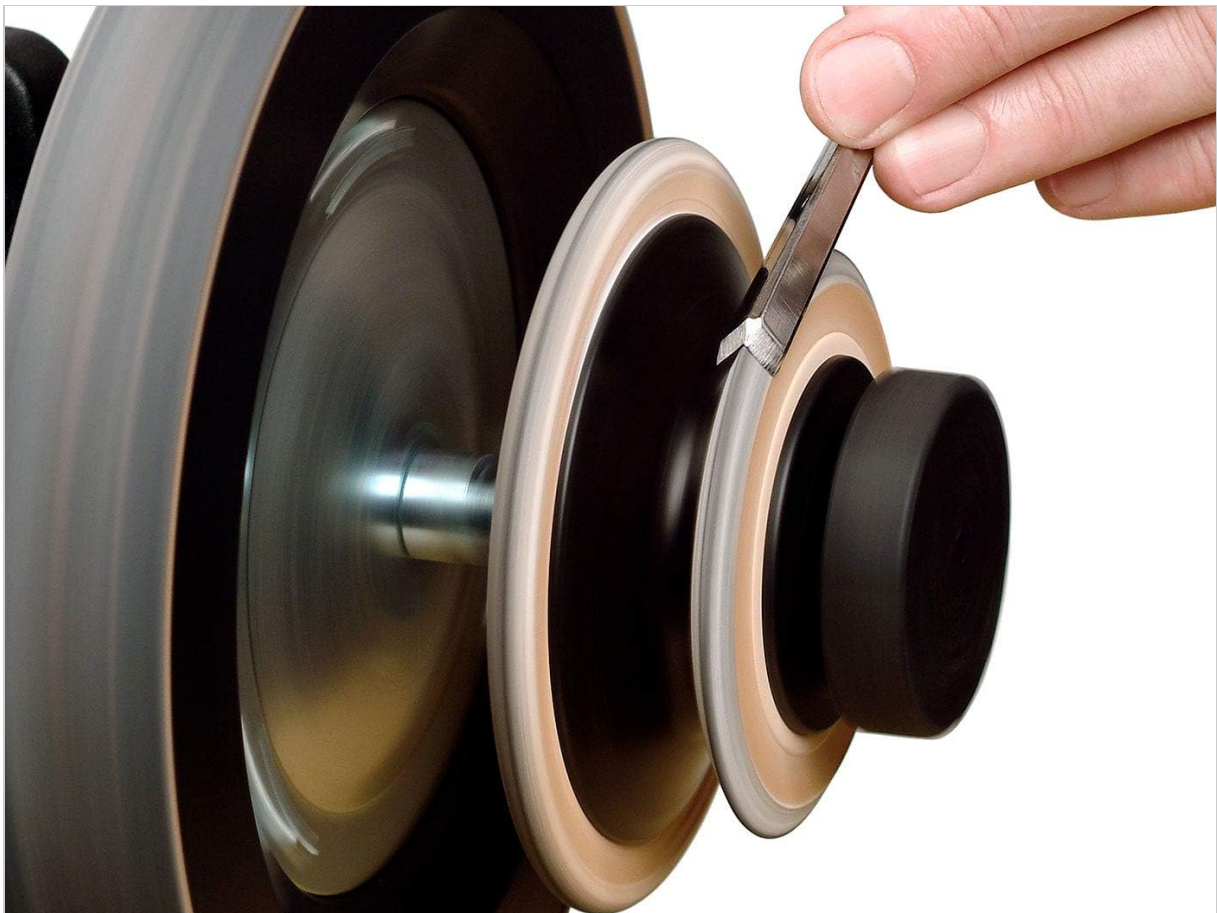
Figure 5.4: A woodturning tool being honed on the Tormek LA-120 Profiled Leather Honing Wheels, achieving a polished, razor-sharp edge.
