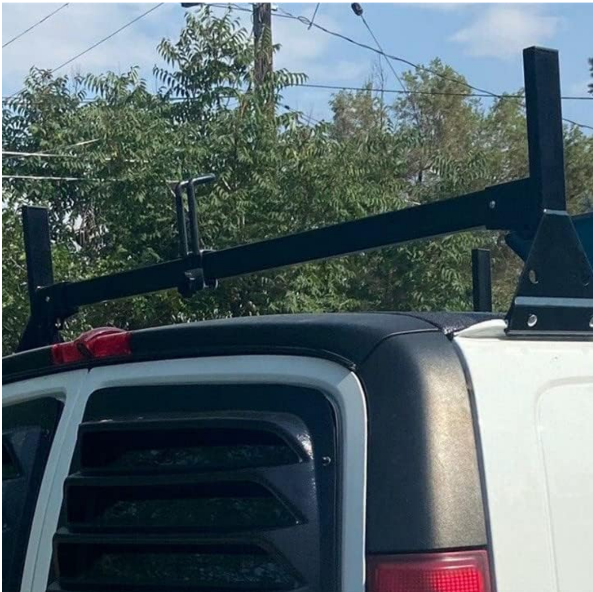
Image 5.1: Rear view of the installed ladder racks on a van.
