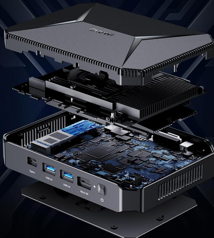
Figure 3: Internal view of the CHUWI Mini PC HeroBox, illustrating the M.2 SSD and the space available for a 2.5-inch SATA drive for storage expansion.
