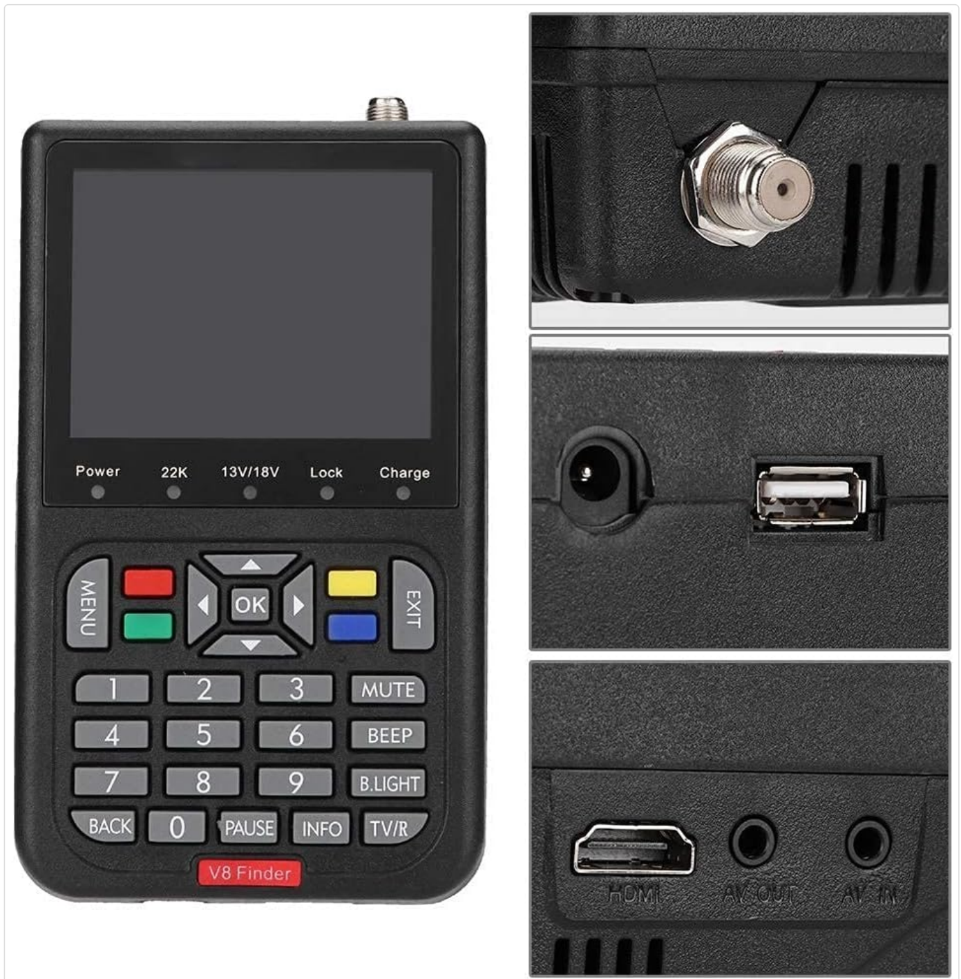
Figure 4.2: Side view illustrating the various ports including LNB IN, USB, DC IN, HDMI, AV OUT, and AV IN connections.
