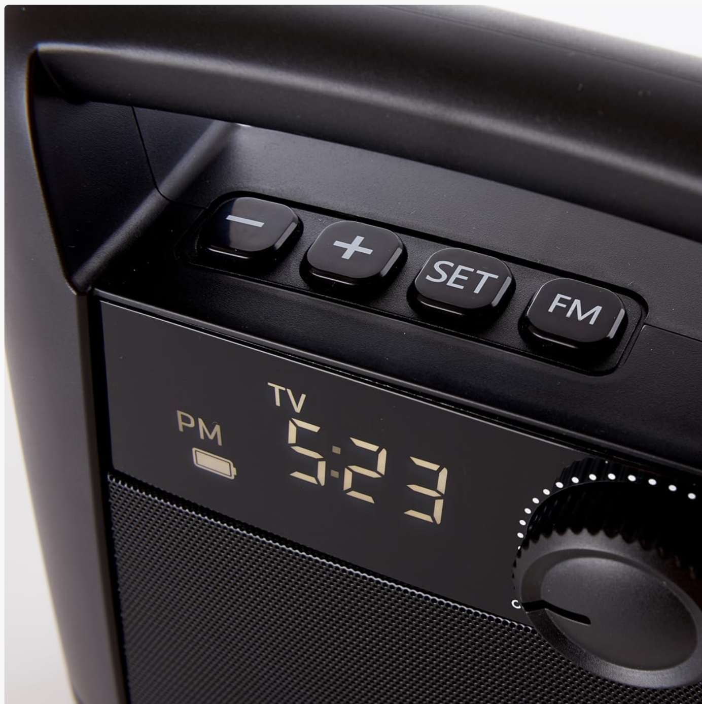
The control panel with volume knob, function buttons, and digital display.
