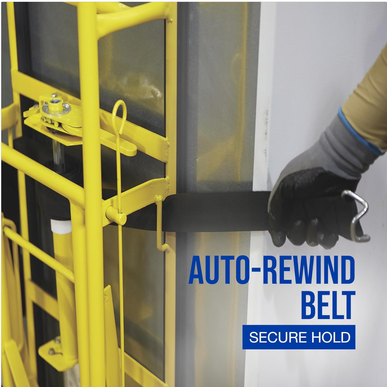
Figure 3.5: The auto-rewind ratchet belt system for securing loads.
