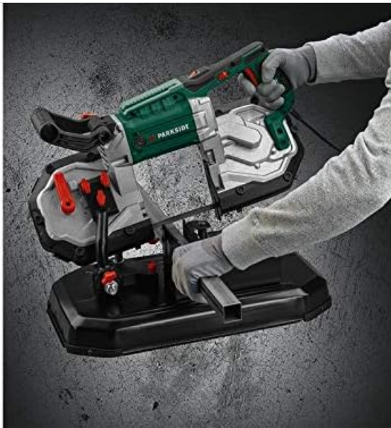
Figure 5.1: An operator demonstrating the use of the Parkside Metal Band Saw in its stationary configuration, cutting a metal profile.
