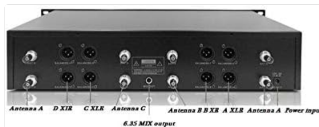
Figure 3.2: Rear panel of the Bolymic 8800S receiver. This view highlights the various audio output ports (XLR and 6.35 MIX output), antenna connections (Antenna A, Antenna B), and the power input. Proper connection of these ports is crucial for system operation.
