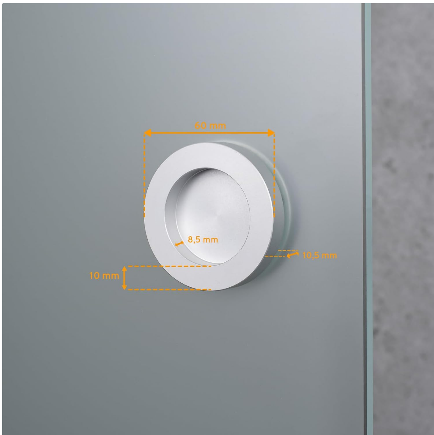
Figure 7: Dimensions of the round recessed handle (69 mm diameter, 8.5 mm depth).
