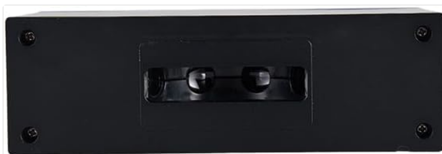
Figure 3.2: Bottom view of the GM-6 Glossmeter, showing the measurement aperture that contacts the surface.
