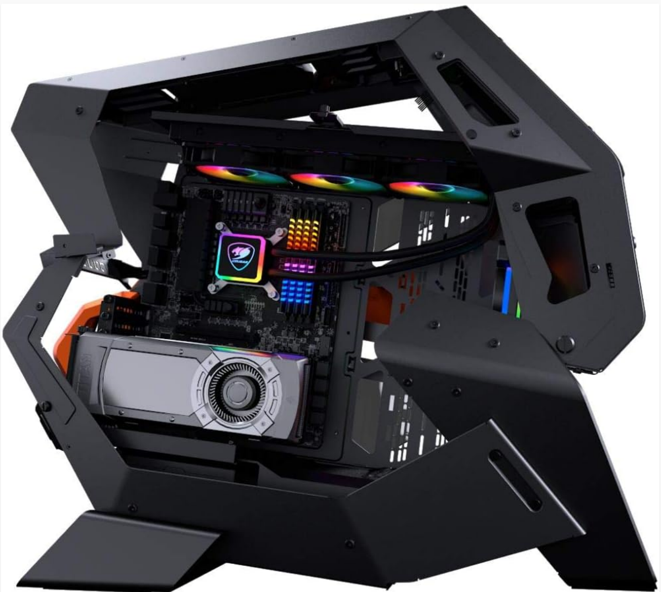
Figure 3.1: The detachable sub-chassis, simplifying component installation.
