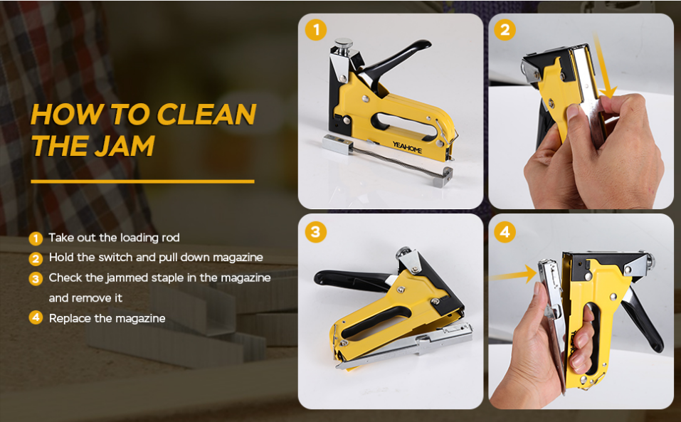
Image 10: Step-by-step guide to clearing a staple jam.
