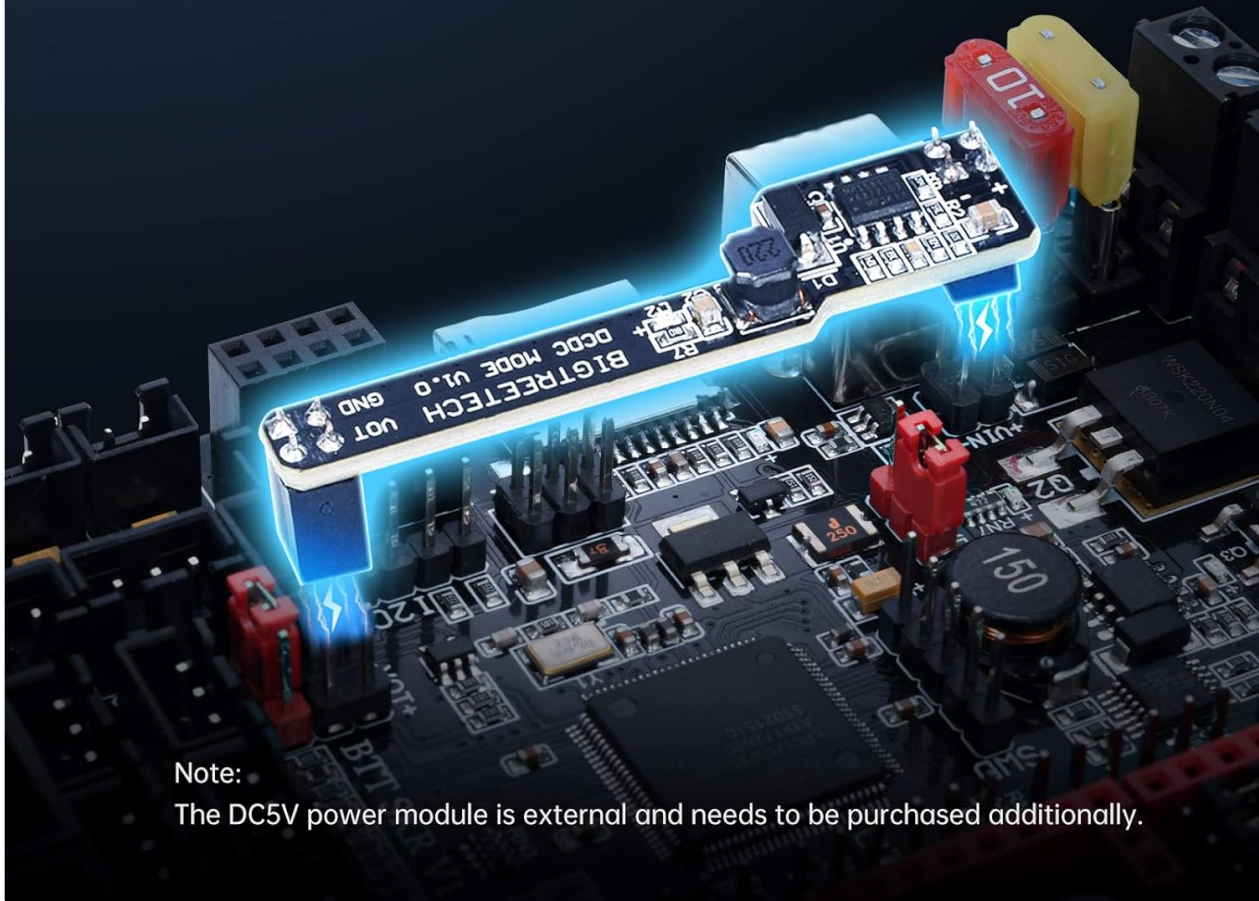
Figure 2.1: DC5V Power Module connection point for TFT, BLTouch, and Neo-pixel.
