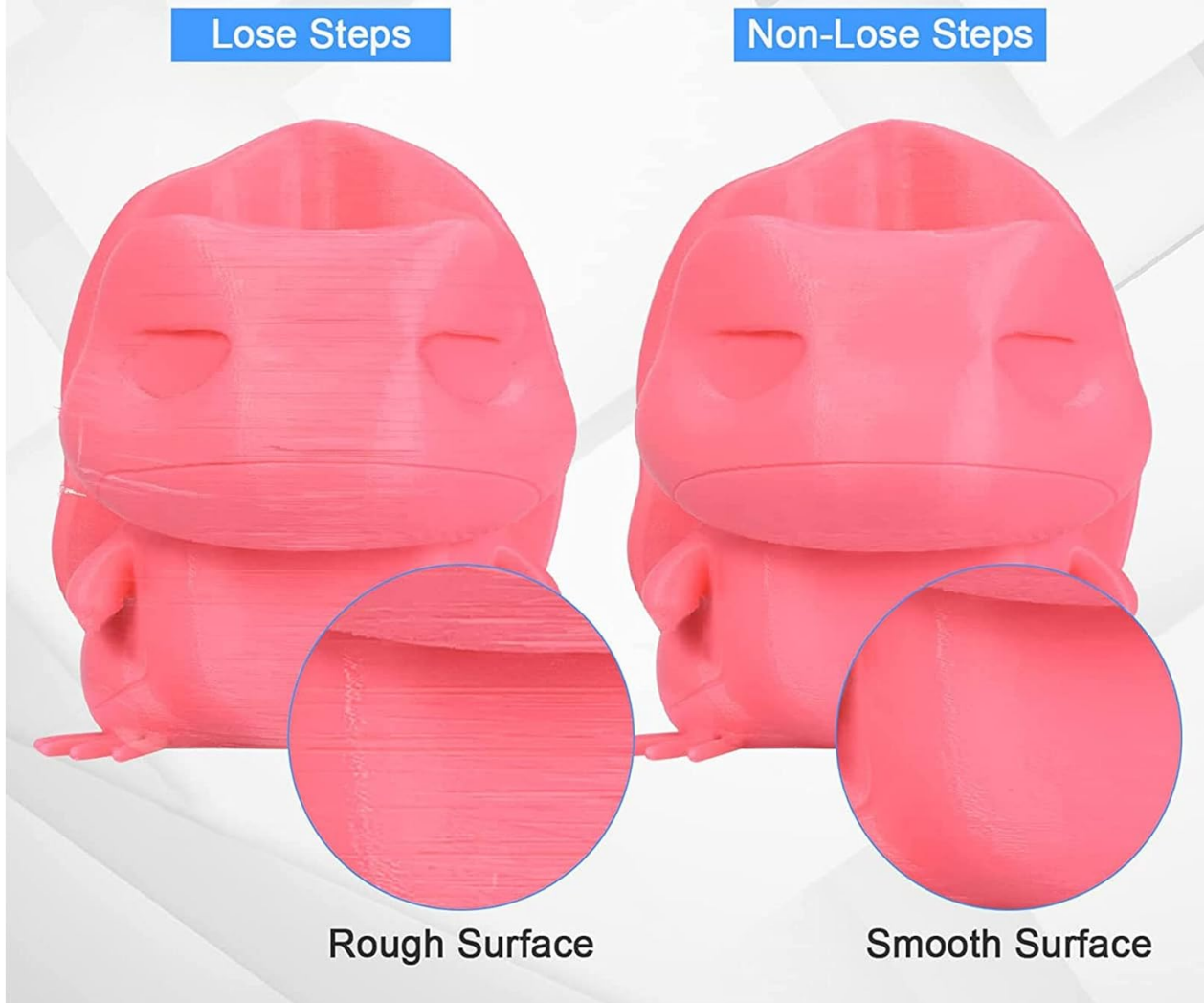
Figure 1.2: Visual comparison of print quality with and without losing steps, demonstrating the precision of the drivers.
