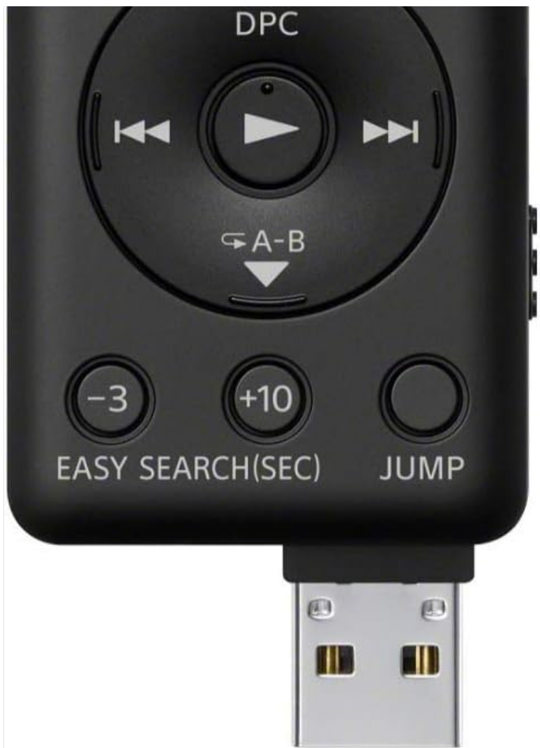
Figure 2.6: Front view with the integrated USB connector extended for direct connection to a computer.
