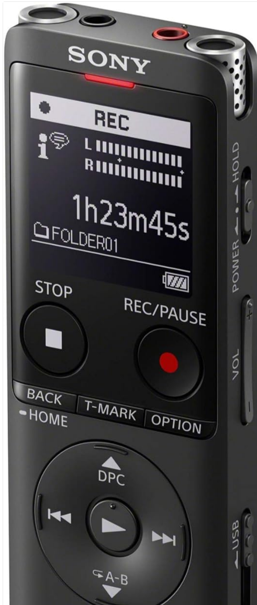
Figure 2.1: Front view of the Sony ICD-UX570 Digital Voice Recorder, showing the display, recording, stop, and playback controls.
