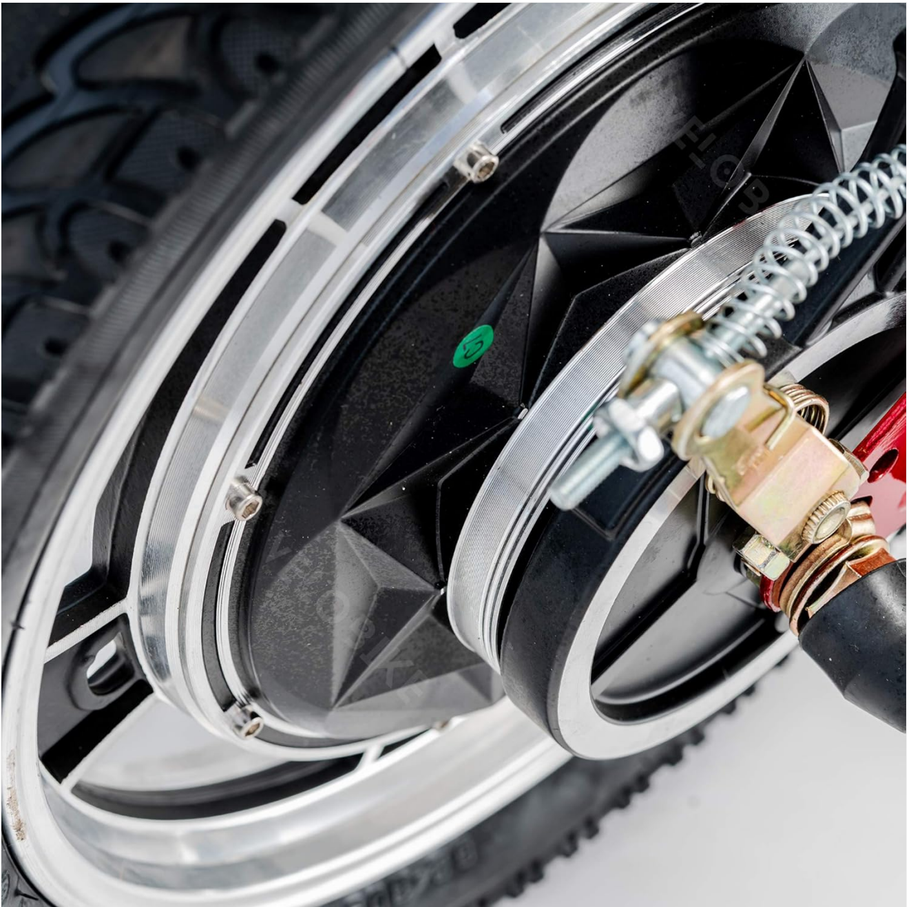
Figure 2.4: Detailed view of the front wheel assembly, including the hub motor and braking mechanism.
