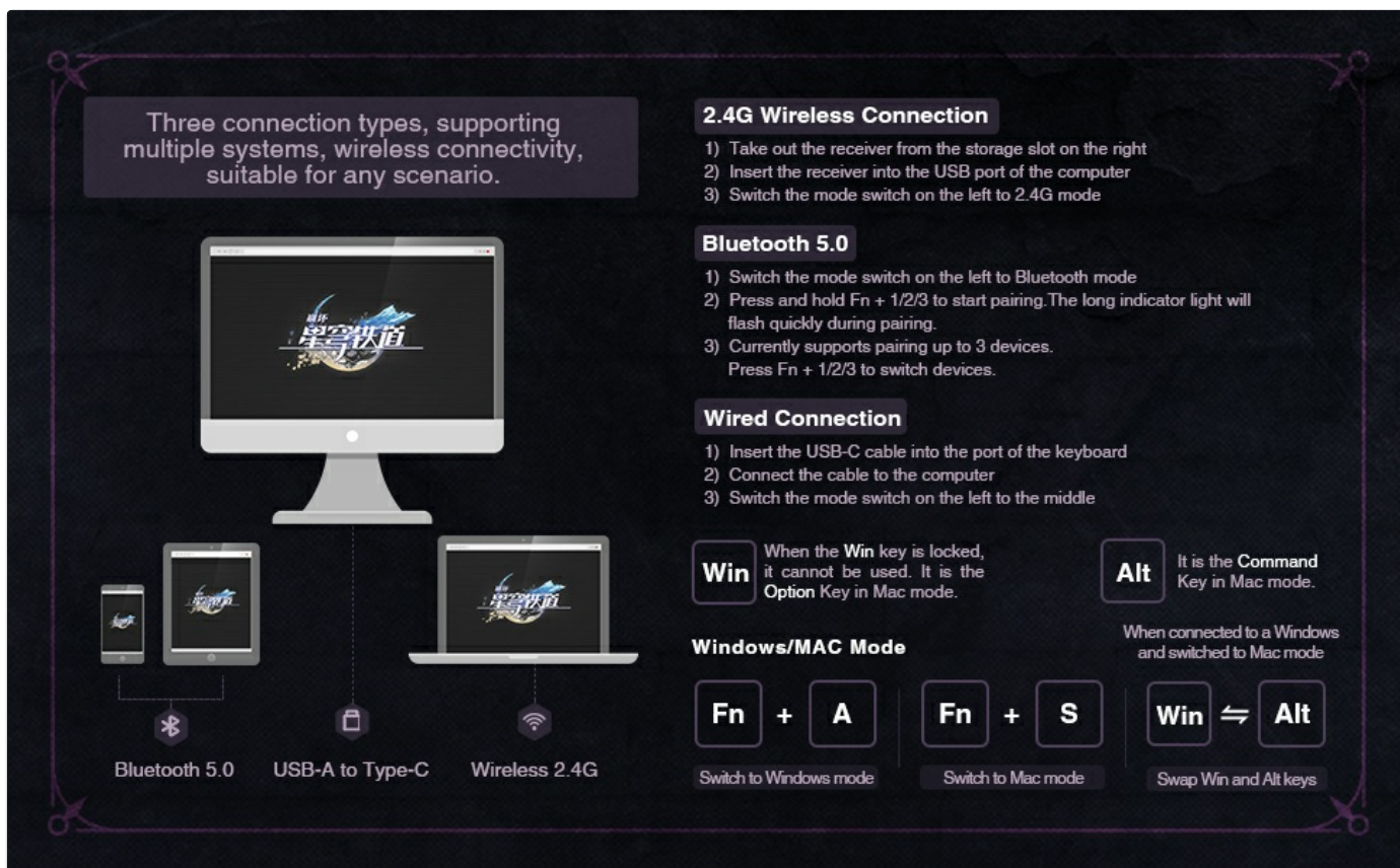
Image: Visual guide for connecting the keyboard via 2.4G wireless, Bluetooth 5.0, and wired USB-C, including system compatibility for Windows and Mac.
