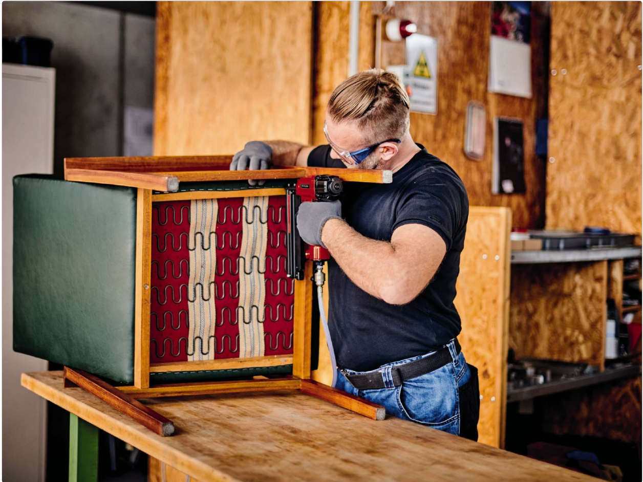
Figure 2: Example of compressor application. This image shows a person using a pneumatic nail gun to attach fabric to a wooden frame, demonstrating a common use for an air compressor in upholstery or woodworking.
