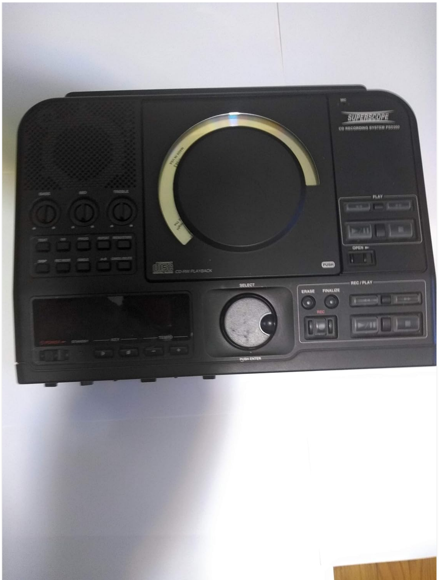
Figure 4.1: Front Panel of the Superscope PSD300. This image displays the main controls including the CD tray, playback buttons, recording controls, and the display screen. On the left are controls for volume, treble, and bass, along with input selection buttons. The central knob is for selection and pushing to enter.
