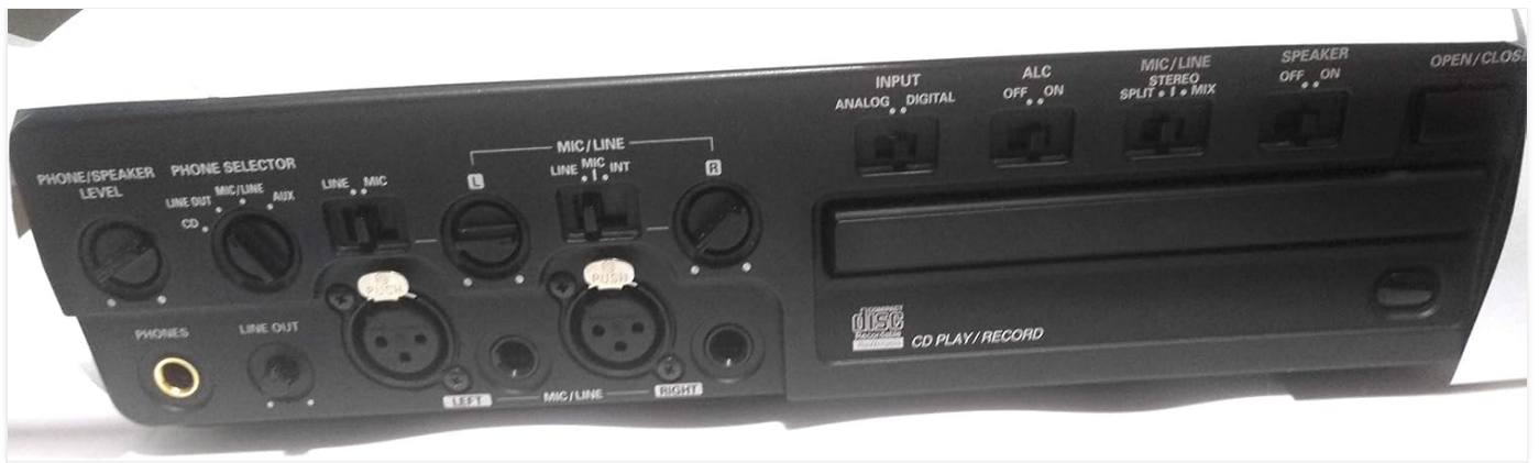
Figure 4.2: Rear Panel of the Superscope PSD300. This image shows the various input and output connections. From left to right: Phone/Speaker Level, Phone Selector (Line/CD, Mic/Line, Aux), Line Out (RCA), Left and Right XLR/TRS combo Mic/Line inputs, Input selector switches (Analog/Digital, Mic/Line, Stereo/Split/Mix), Speaker On/Off, and Open/Close for the CD tray.
