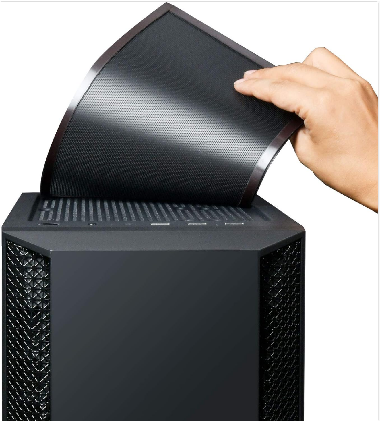
Figure 7: Removing Top Dust Filter
