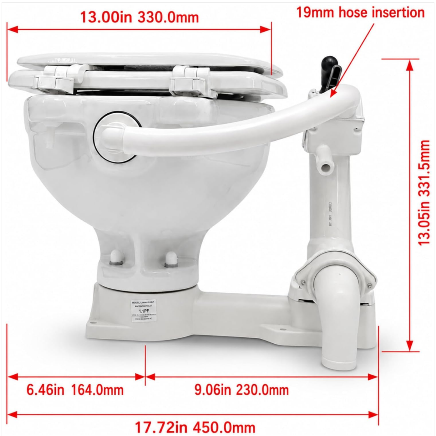
Figure 2: Detailed dimensions of the SFMTM-01 marine toilet.
