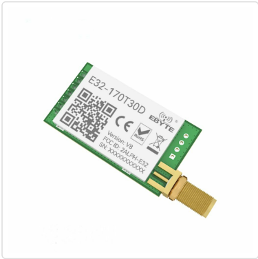
Figure 1: Top view of the EBYTE E32-170T30D LoRa module, showing the EBYTE logo, model number, QR code, CE, RoHS, and FCC ID markings, along with the SMA antenna connector.
