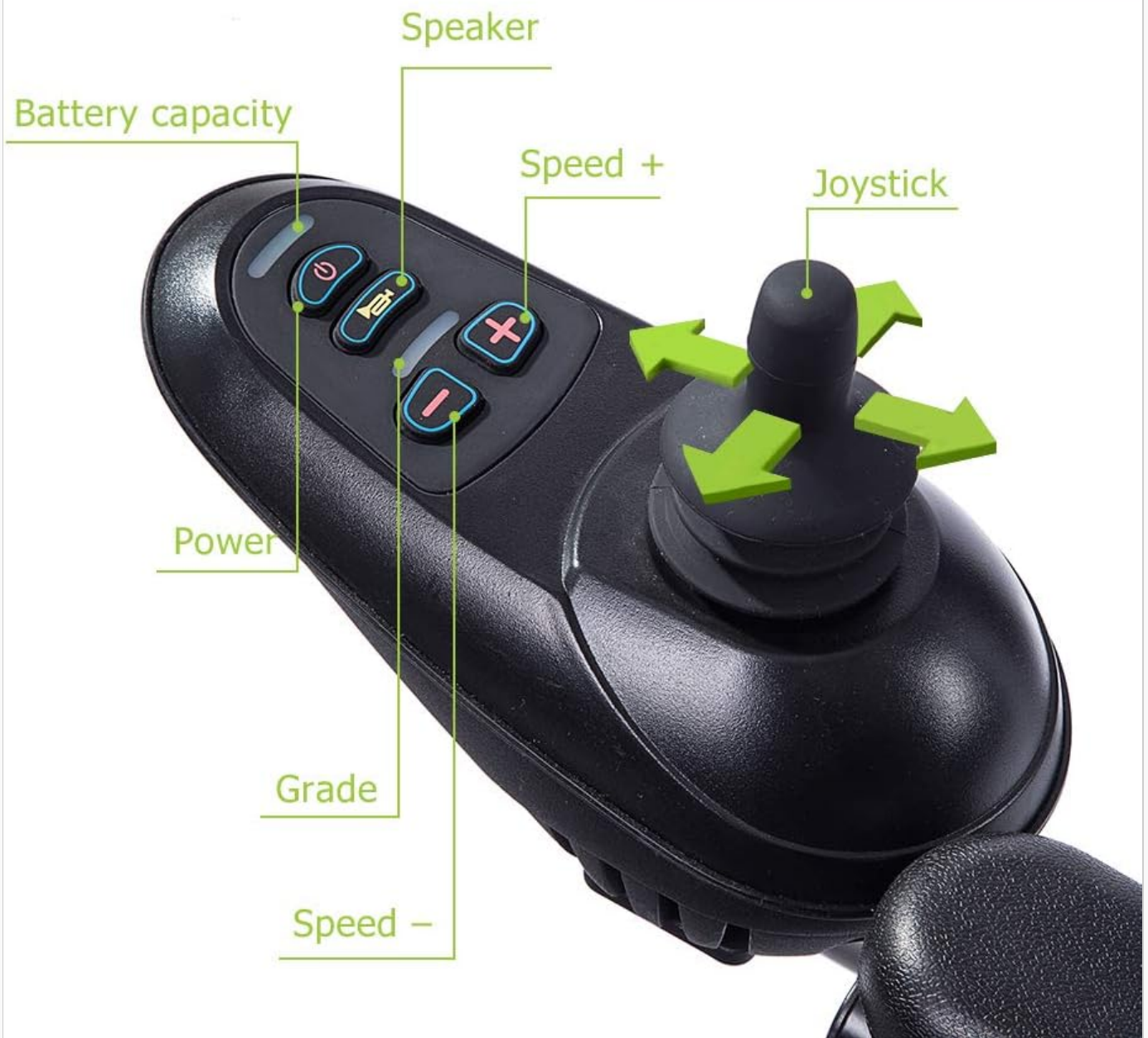
Image 5.1: Detailed view of the joystick controller with labeled functions for easy operation.
