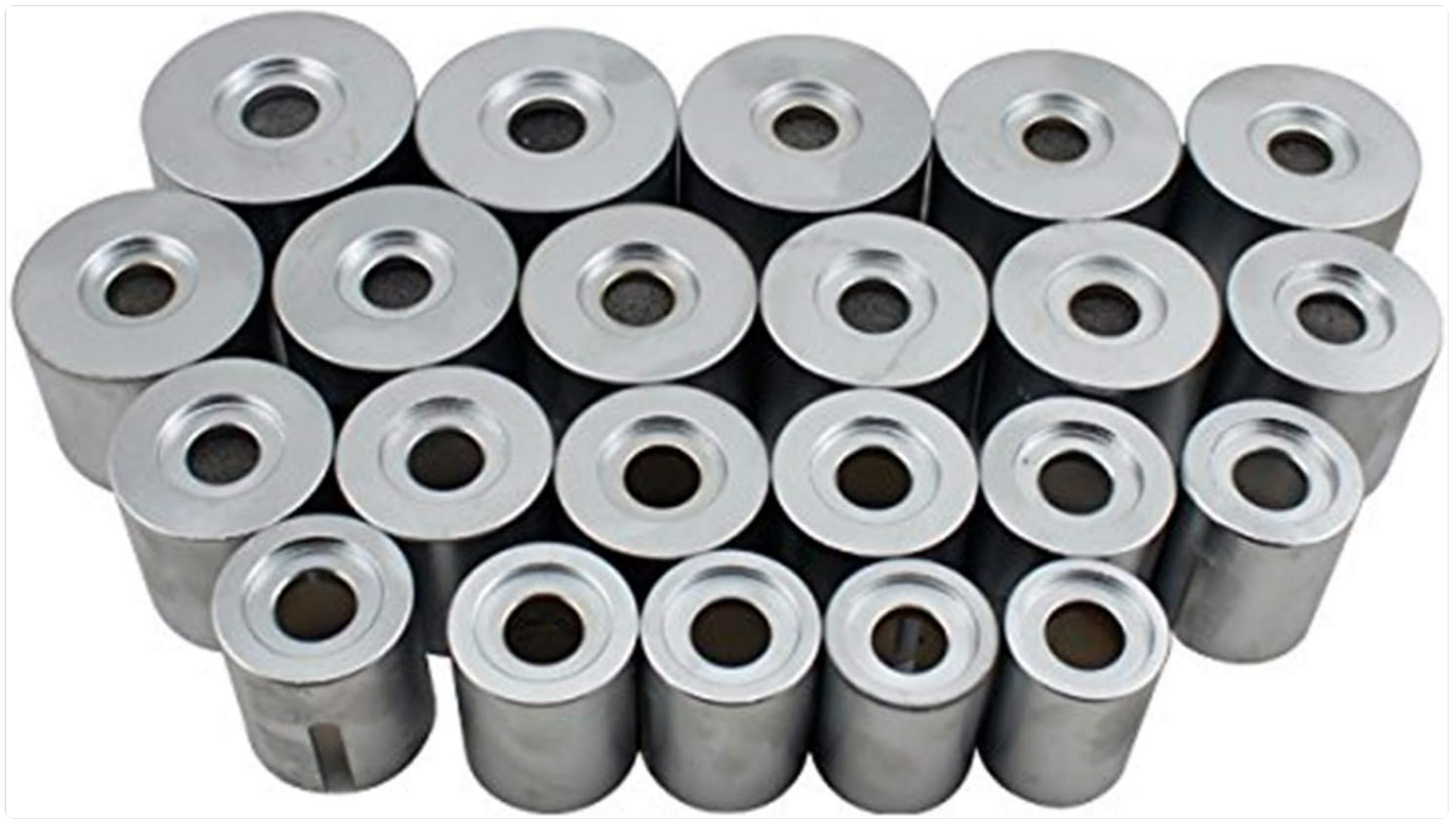
Figure 3.3: Collection of 22 Pressure Pieces. This image shows the 22 cylindrical pressure pieces, also known as sleeves or adapters. These pieces come in various inner diameters (34–80mm) and outer diameters (44–90mm) to fit a wide range of bushings and bearings.
