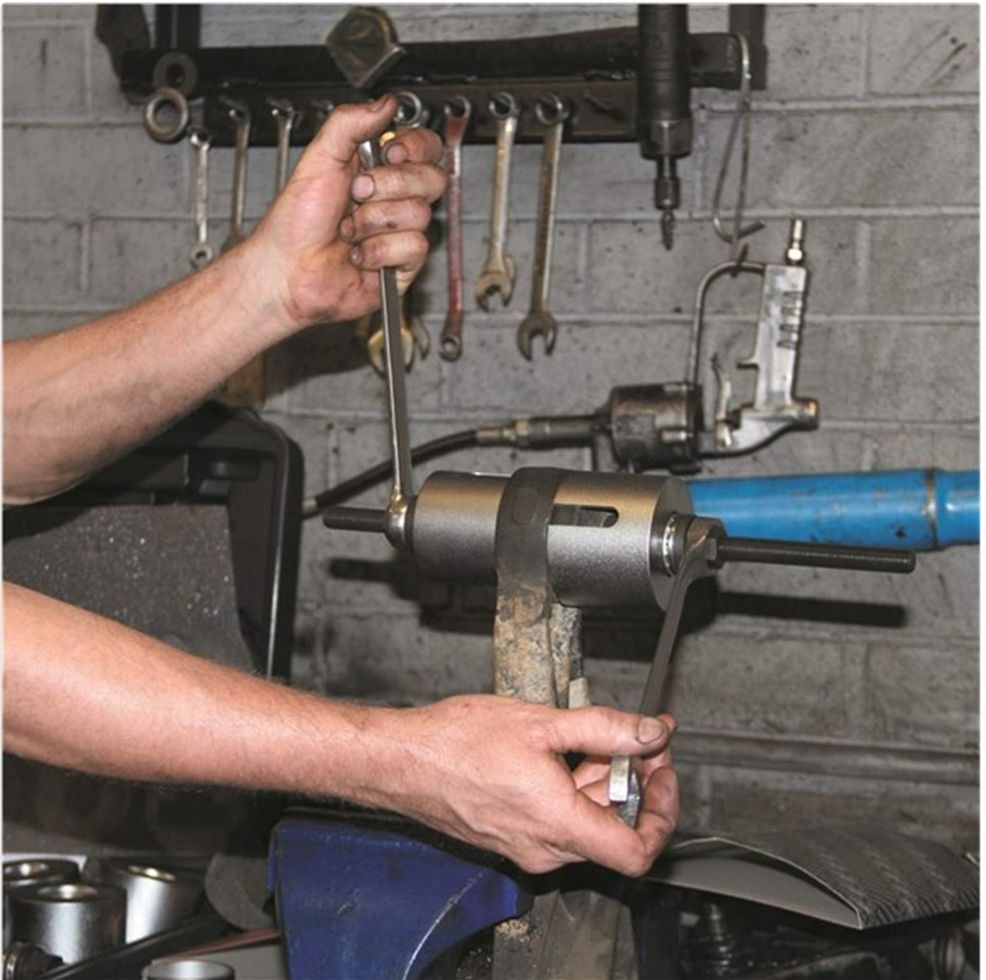
Figure 5.1: Tool in Operation. This image illustrates the tool being used to press out a component. Two wrenches are applied to the nuts on the spindle, demonstrating the manual force application required for the operation. The component is secured in a vise.
