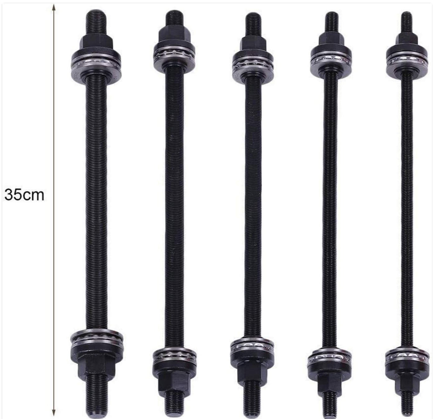
Figure 3.2: Set of 5 Spindles. This image displays the five robust threaded spindles, ranging in size from M10 to M18. Each spindle is equipped with nuts and thrust bearings for smooth operation. One spindle is shown with a measurement indicating its length of 35cm.
