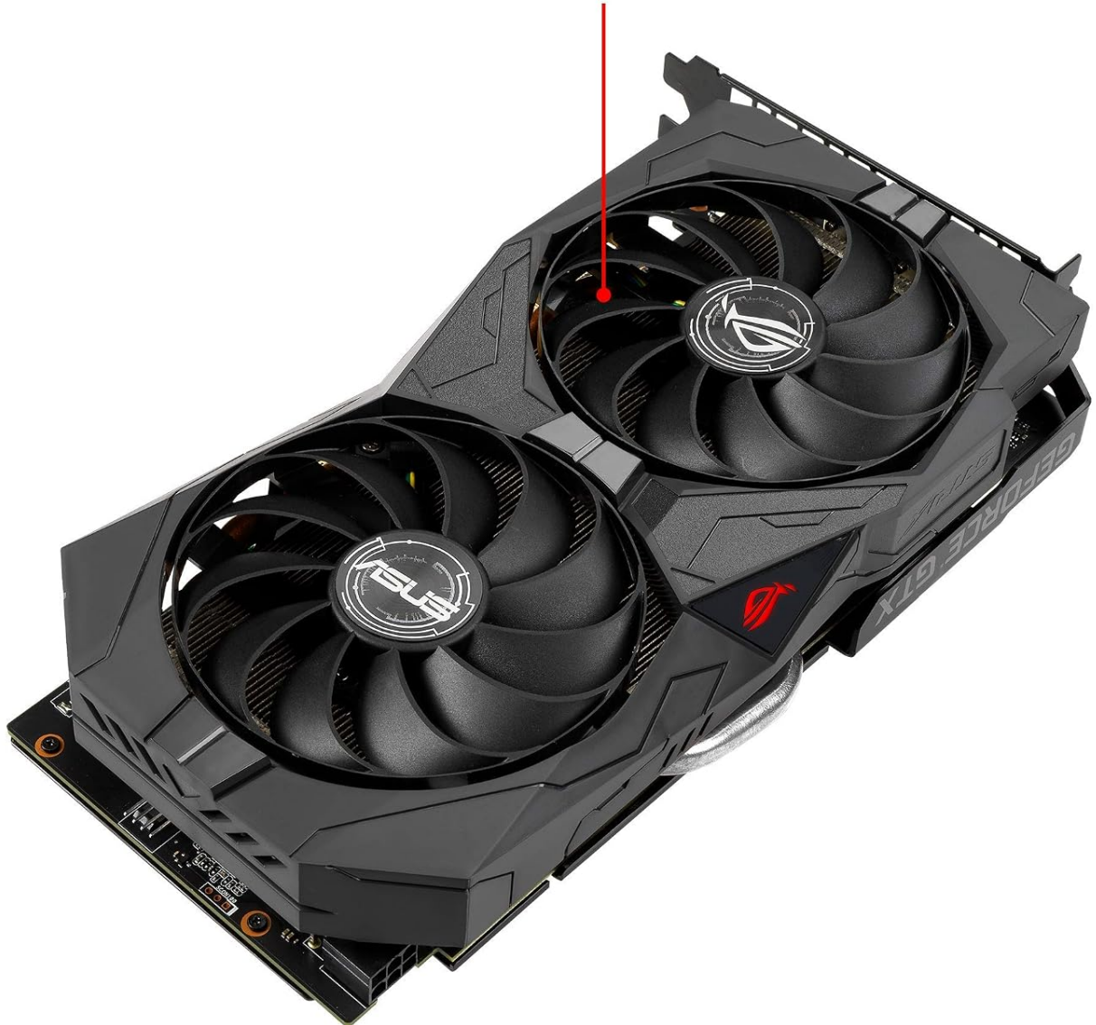
Figure 3: The Axial-tech fan design, featuring a smaller fan hub for longer blades and a barrier ring to increase downward air pressure, which aids in efficient cooling.
