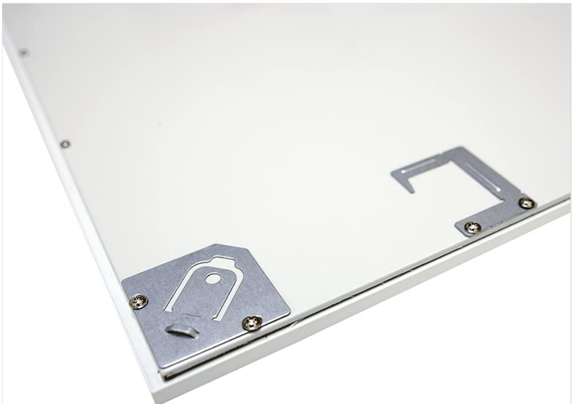
Image: Integrated grid retention clips. These clips are designed to secure the panel within a T-bar ceiling grid.
