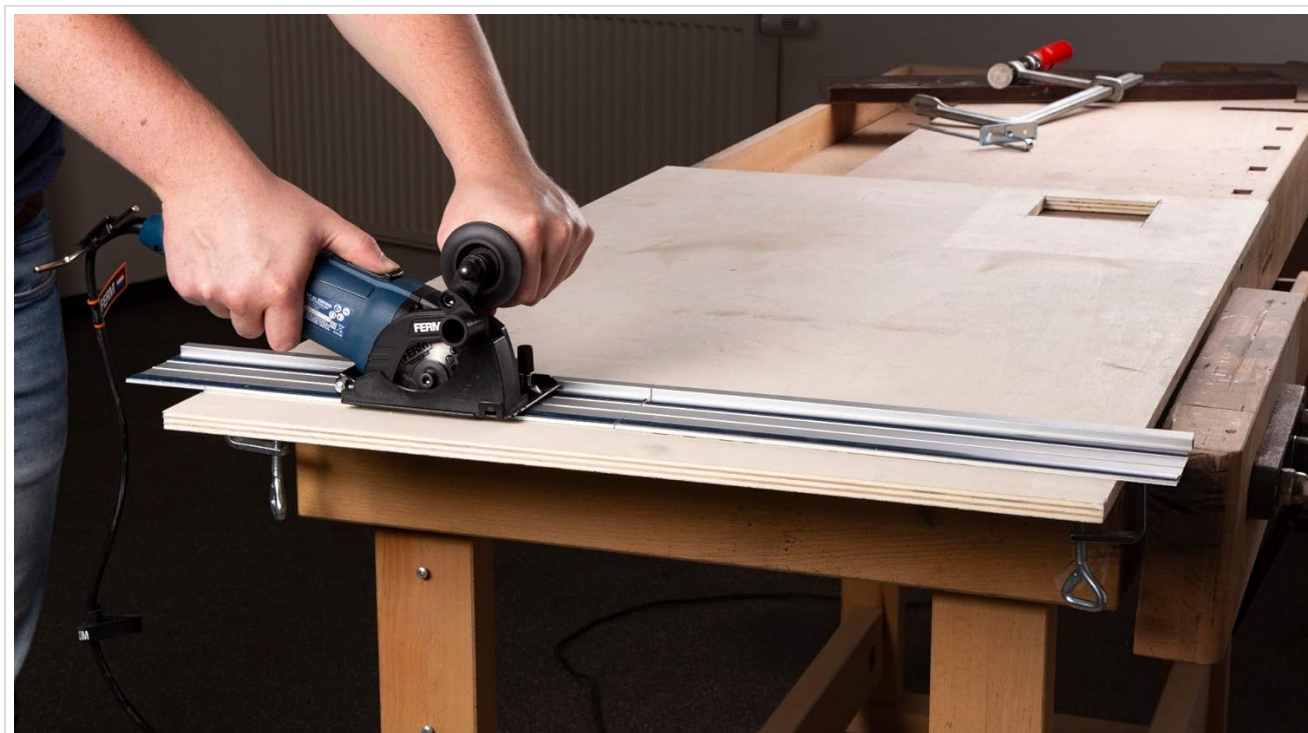
Image: A broader perspective of the FERM Precision Circular Saw in action, showing the setup with guide rails clamped to a workpiece on a workbench.
