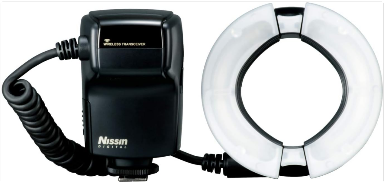
Image: Overview of the Nissin MF18 Macro Ring Flash and its included components, including the main flash unit, ring flash head, and various adapter rings.
