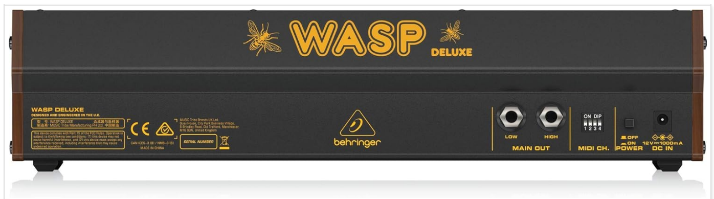
Figure 2: Rear panel of the Behringer WASP DELUXE, showing the power input, audio outputs, and MIDI/USB ports.
