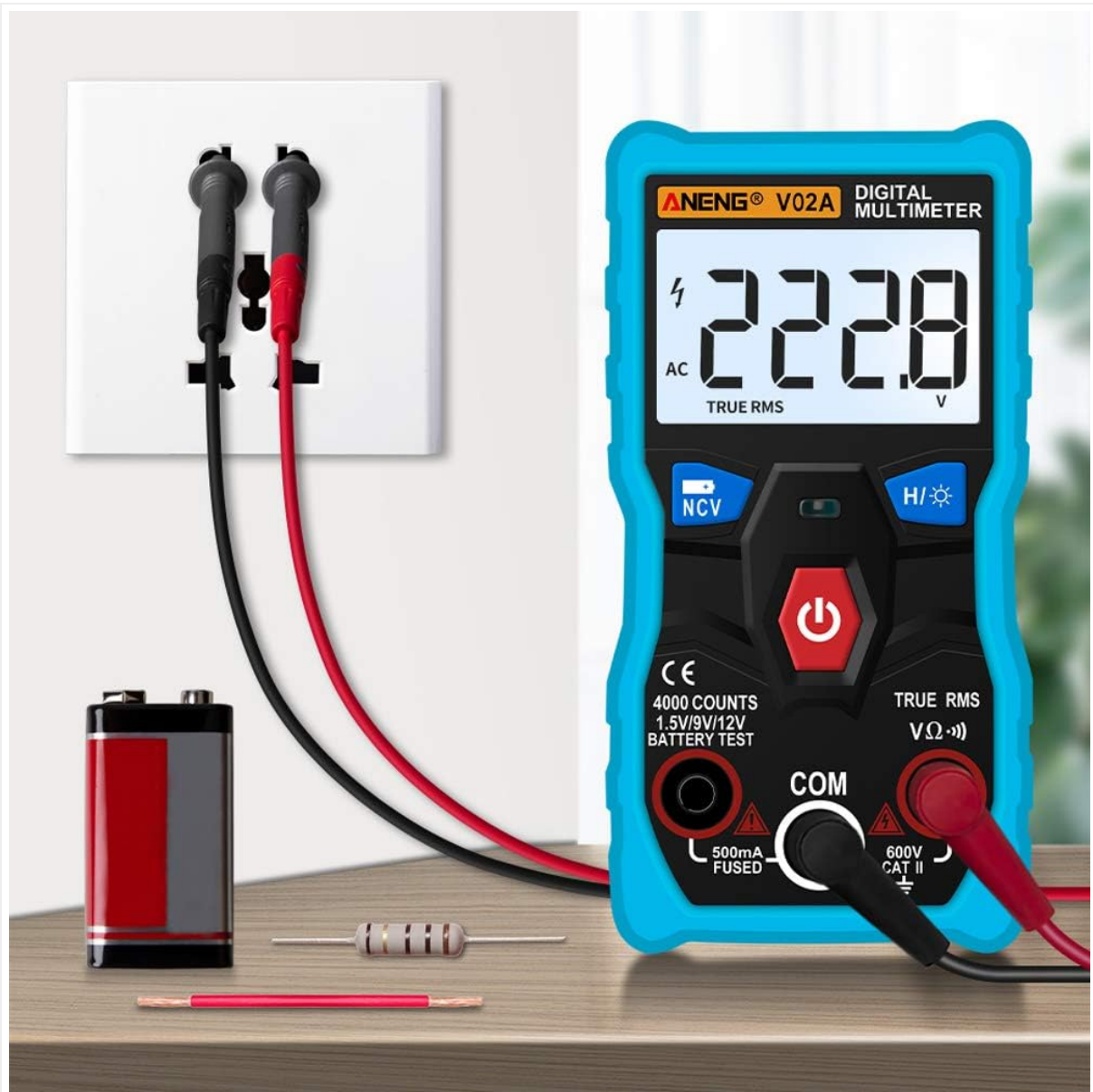
Figure 4.1: The multimeter connected to an AC outlet to measure voltage.
