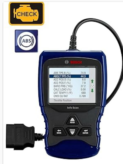
Image 2.2: The Bosch OBD 1150 Scan Tool connected to its OBD-II cable.
