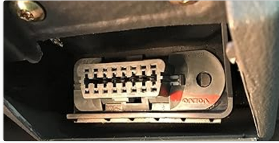
Image 2.1: Standard location of a vehicle's OBD-II diagnostic port.
