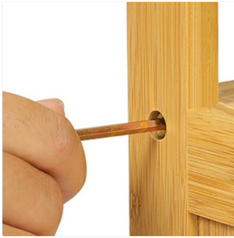
Image: A hand tightening a screw with a hex key during assembly.
