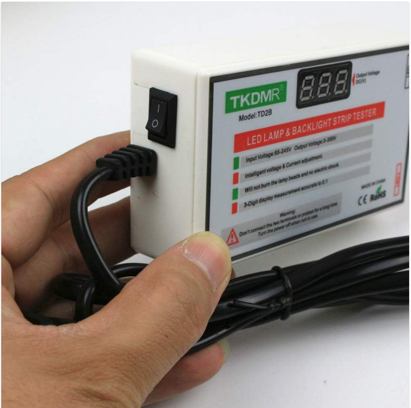
Image 3.2: A hand demonstrating the operation of the power switch on the side of the TKDMR LED Lamp Bead TV Backlight Tester.
