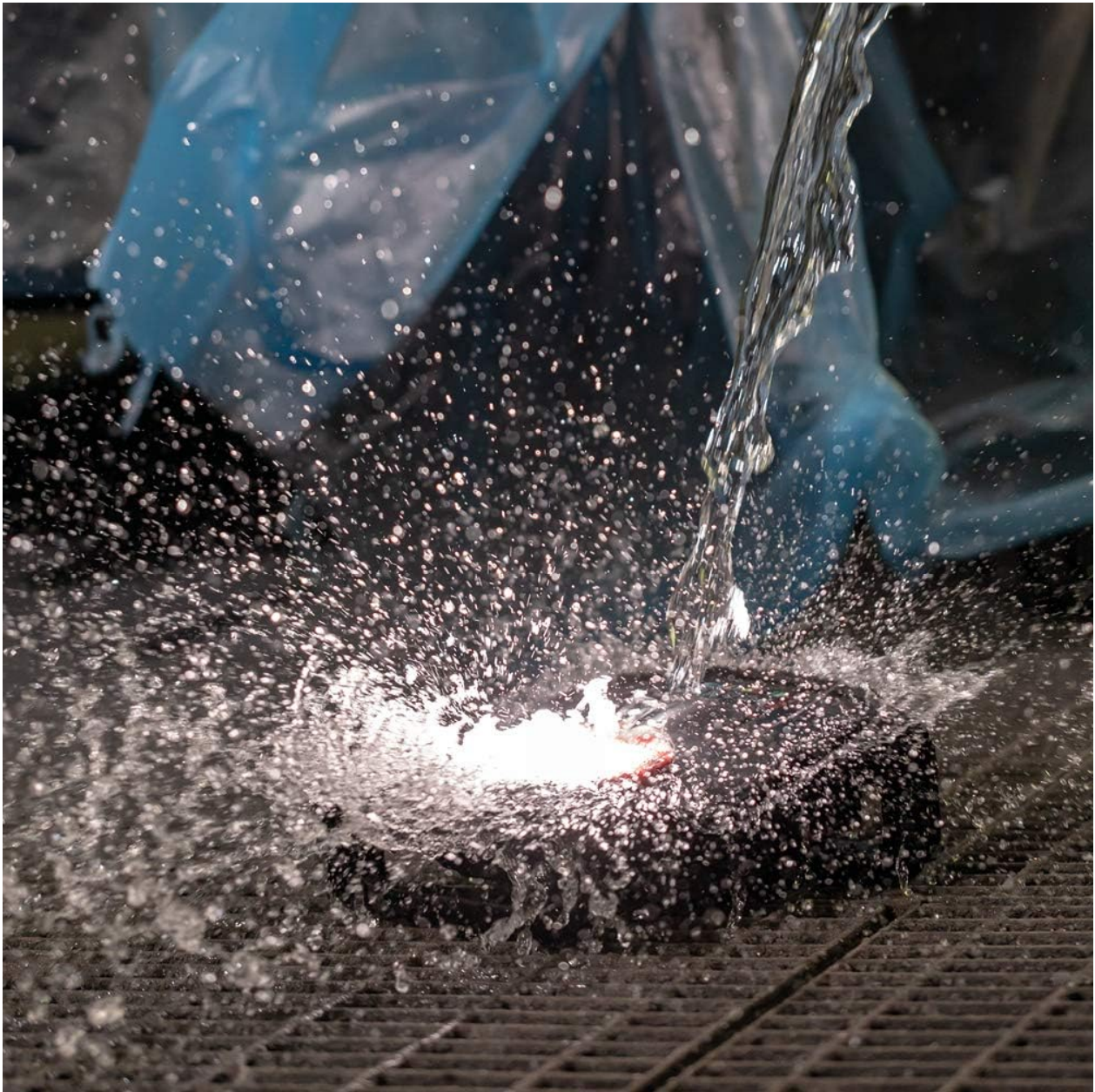
Figure 4: Water resistance of the MULTIMATCH 8. This image shows the light being sprayed with water, indicating its durability and IP67 rating.
