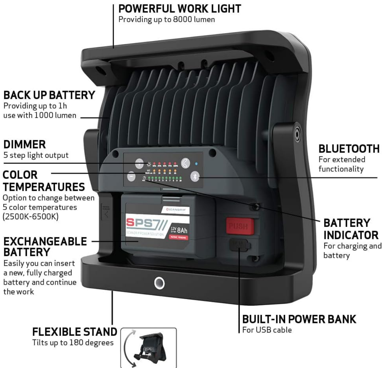
Figure 1: Overview of SCANGRIP MULTIMATCH 8 features. This image shows the back of the light with labels indicating the powerful work light, backup battery, dimmer, color temperatures, exchangeable battery, flexible stand, built-in power bank, battery indicator, and Bluetooth functionality.
