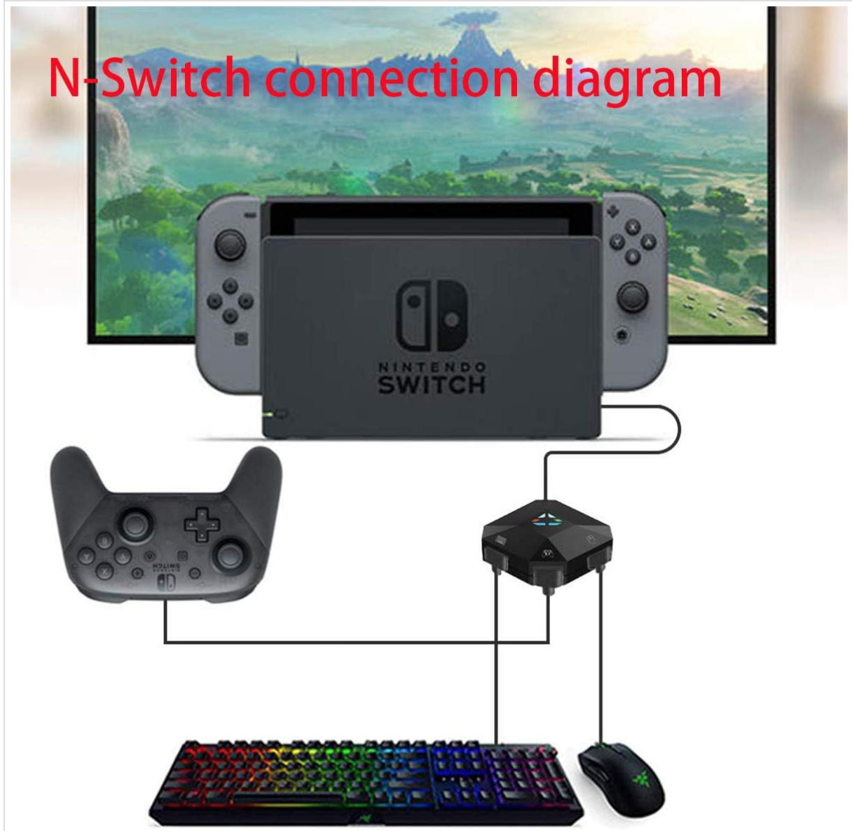
Image 3.2: A visual guide demonstrating the connection of the TNS-19077 adapter to a Nintendo Switch console, along with a keyboard, mouse, and a wired Pro Controller.
