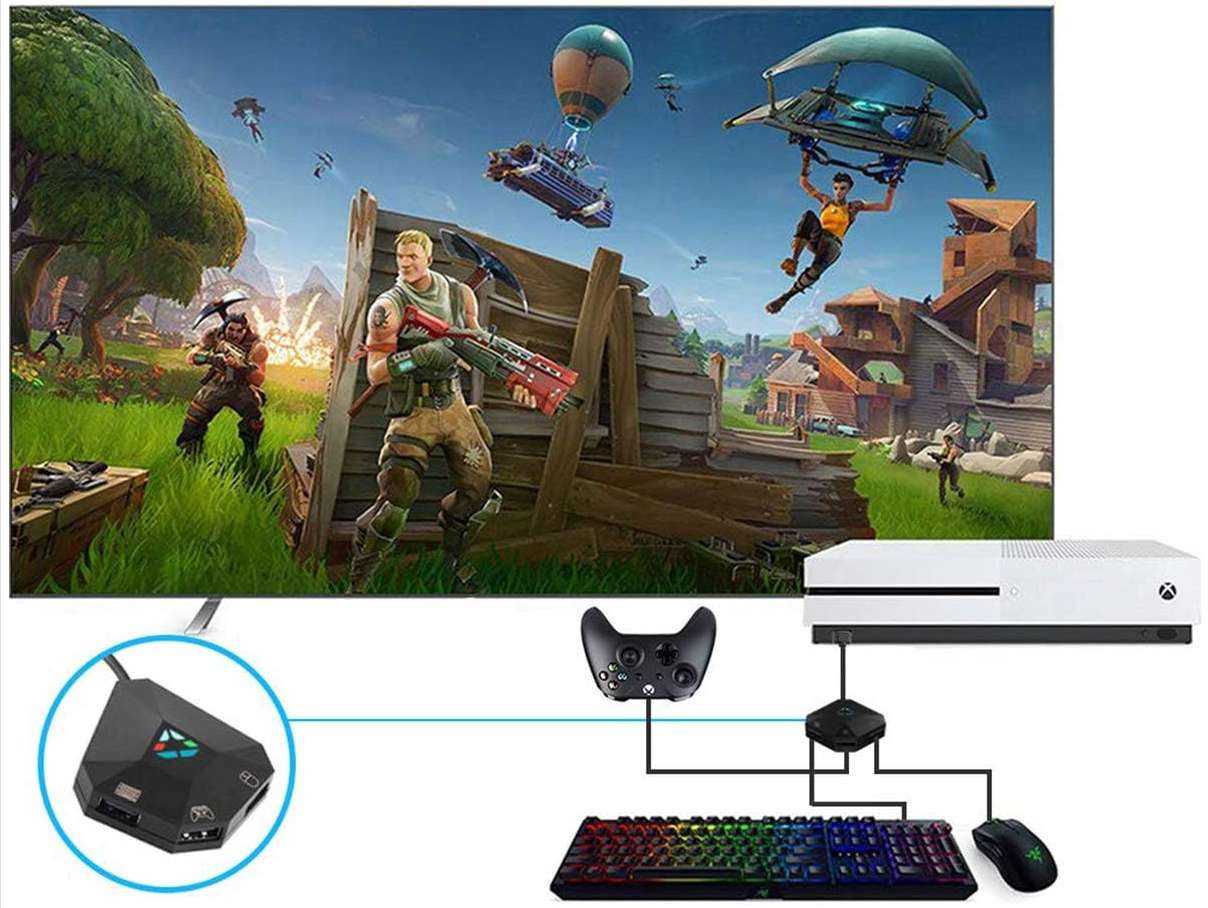
Image 3.4: A diagram illustrating the connection of the TNS-19077 adapter to an Xbox One console, showing the required original Xbox One controller, keyboard, and mouse connections.
